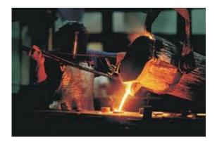
A worker was seriously injured while removing molten metal from a slag pit. A steam explosion occurred when molten metal made contact with water that had accumulated in the pit area. The employer pleaded guilty to failing to ensure that work performed in the removal of molten metal from a slag pit was performed in a safe manner. It was fined \$93,800 [Gerdau Ameristeel Corp., Govt. News Release, Sept. 4, 2014].
