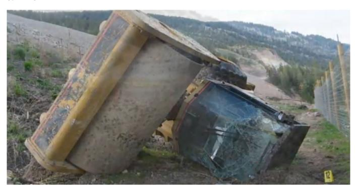
Many workplaces use various kinds of powered mobile equipment, such as forklift, backhoes, etc. This equipment can obviously endanger workers around it if the operator'and the workers'aren't alert and careful. For example, it can run over an unaware worker who strays into its path. But such equipment can also endanger its operators, especially if it tips or rolls over.
