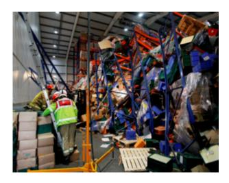
These storage racks collapsed and buried a worker underneath hundreds of pounds of cheese and metal shelving. How could this incident have been prevented'
