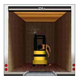
Many workplaces use equipment and tools powered by gasoline, diesel, propane and the like. If such equipment is used in an enclosed space and without adequate ventilation, it can put workers in grave danger.
