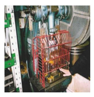
This mechanical power press has a guard. But how effective is the guard at protecting workers'
