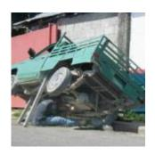
Imagine the consequences for this worker if either of these boards was knocked over or fell'
