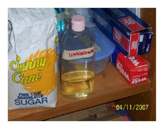
The answer, of course, is not a proper WHMIS label. And while it may be better than no label at all, this makeshift 'UNKNOWN' tag is appallingly inadequate'especially when you consider that this photo comes from a chemical laboratory.
