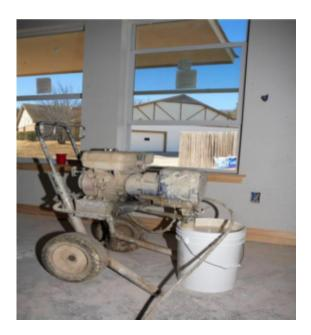
This paint sprayer is being used to paint this room, but it's not designed to be used indoors. Why could such use be hazardous'
