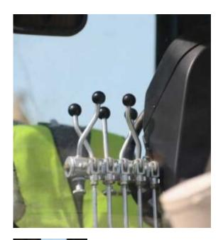
This alert from the Ontario MOL warns of a potential hazard involving exposed crane controls on crane trucks.
