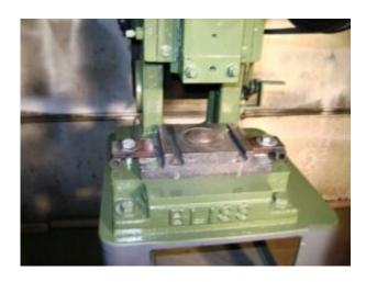
Three fingers on a worker's left hand were severed when a punch press machine top plate activated and pressed down on his fingers. The company failed to ensure the punch press had safeguards installed to prevent workers from having contact with hazardous points of the machine. It pleaded guilty under Sec. 16.5(1)(b) of the Workplace Safety and Health Regulation to a guarding violation and was fined \$60,050 [Cadorath Plating Co. Ltd., Govt. News Release, July 18, 2012].
