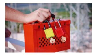
Companies have a duty to protect workers both while using equipment and machinery for their intended purpose and when repairing and maintaining that equipment. The primary way of fulfilling that duty is through what's called 'lockout,' which is when a equipment has been turned off and rendered inoperable with the use of a lock. But sometimes so-called 'group lockout' is more appropriate than standard lockout given the circumstances.
