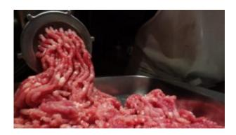
A worker cleaning a machine suffered serious injuries after getting his hand caught in its rotating piece. WorkSafeBC inspectors found that there had been a guard in place but that somebody removed it to make it easier to clean the machine. To make matters worse, the machine was new and the victim didn't receive training on how to use it safely. Result: The employer was hit with a \$97,847 penalty for 2 OHS violations [Punjab Milk Foods, May 15, 2020].
