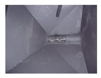
A worker was killed when his hand was caught between a moving upright auger and the power take off shaft of an extractor. His employer pleaded guilty to failing to provide an effective safeguard where a worker may contact a dangerous part of a moving machine and was fined \$21,000 [Greenspring Ag Services Ltd., Govt. News Release, Oct. 23, 2013].
