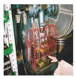
A worker was using a wire stripper machine to remove the insulation off of scrap wire. While feeding wire into the stripper, his left hand came into contact with the machine's feeding rolls. He sustained serious lacerations to two fingers. The company pleaded guilty to failing to have safeguards on the wire stripper machine and to provide adequate supervision of its workers. The court fined it \$18,800 [Rakowski Cartage and Wrecking Ltd., Govt. News Release, Oct. 22, 2014].
