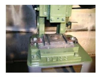
A worker was trimming metal bars using an eccentric punch press. While removing a piece of metal from the press, it activated, pinching the worker's left hand and amputating two fingers. The employer pleaded guilty to failing to provide a worker with the CSA standards on the operation and safeguarding of power press machinery and to ensure that the press was regularly inspected. The court fined it \$35,000 [Buhler Trading Inc., Govt. News Release, Jan. 13, 2015].
