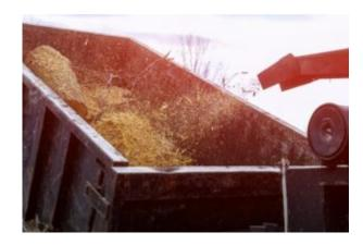
Wood chippers are often used this time of year to chop up fallen branches' and to turn Christmas trees into mulch after the holidays. Tree branches and trunk sections fed manually into the machine's infeed hopper are grabbed by the feed mechanism or chipper knives, which cut and propel wood chips through the discharge spout. So clearly this equipment can be very dangerous if not used properly.
